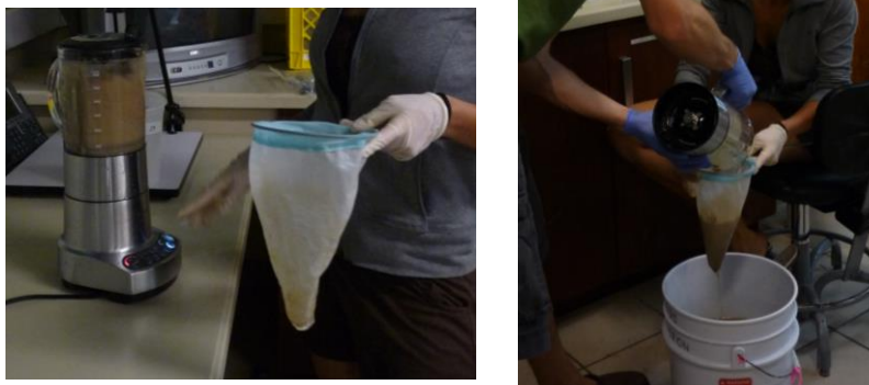
Figure 12. Blend of the scraped fraction. During 5 seconds with a proportion 1:1 sample:ethanol. After blending, pour the blend back into a nitex net and rinse with ethanol (several times).
