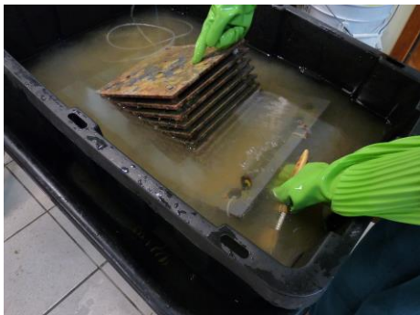
Figure 4. Disassemble the ARMS and brush the plates separately, as they are disassembled.
