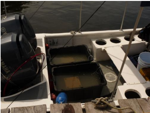
Figure 3. ARMS stored in action packer for carrying them in the boat, with sea water and aeration. Cover the container when possible.
