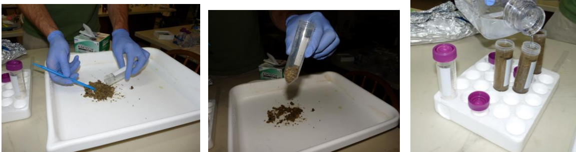
Figure 13. After squeezing out the liquid, place the sample into 50 ml falcon tube up to 10 ml, fill with DMSO and shake vigorously.
