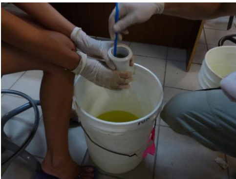
Figure 8. Rinse the sample with ethanol through 2-piece plastic tube with a piece of nitex.
